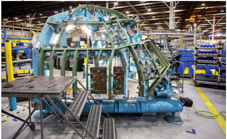
Cockpit structure of the first C-130J-30 airframe earmarked for conversion to E-130J standard in production at the Lockheed Martin plant in Marietta, Georgia. (Image credit: David L. Key/Lockheed Martin)
