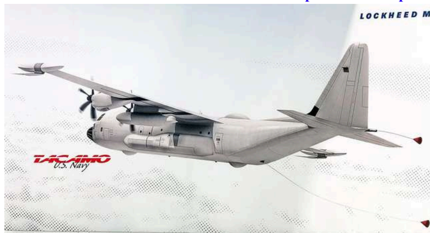
An artist's impression of the E-130J as it will appear in service, showing two trailing wire antennas for low frequency communications and a variety of radomes and communications equipment on the fuselage. (Image credit: Lockheed Martin via TWZ)
